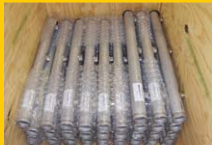
These assemblies are modular and can be shipped economically via common transport. The units are field-assembled easily using Victaulic coupled connections.
